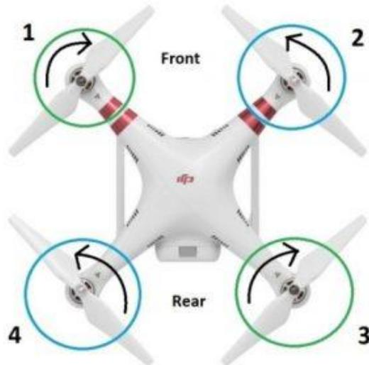
Each pair of opposite rotors is turning the same way. One pair is turning clockwise and the other is anticlockwise
