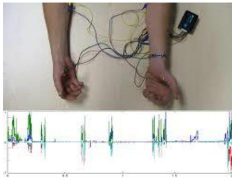
Fig. 3. Electric potential measurement at wrist
