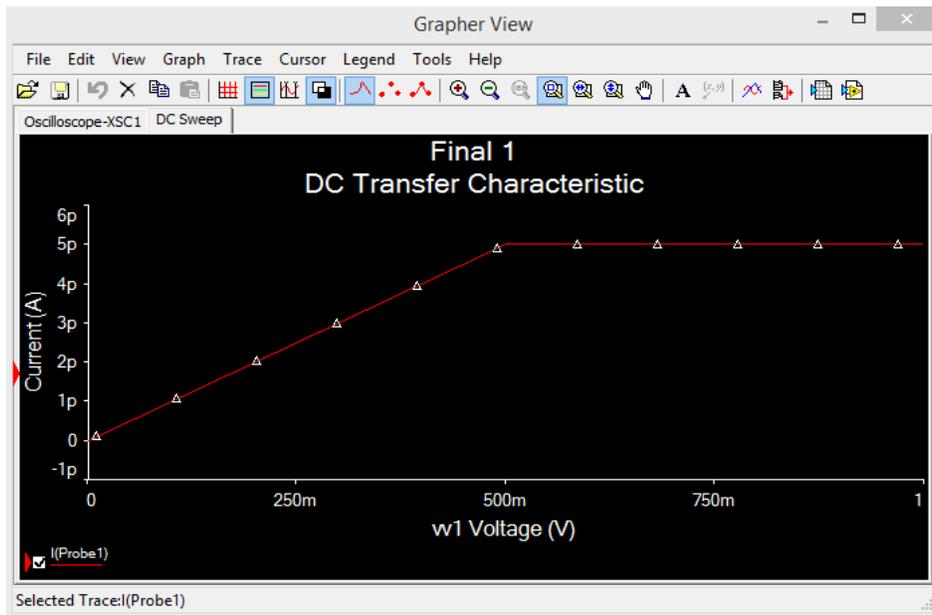
Fig. 8. DC Transfer Characteristics
