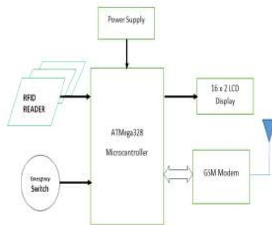
Figure 1. Block Diagram
