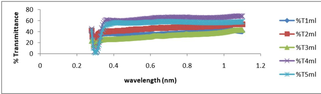
**Figure 4.0:** graph of % transmittance vs. wavelength (nm) for PbSe thin films deposited at 27°C varying pH
