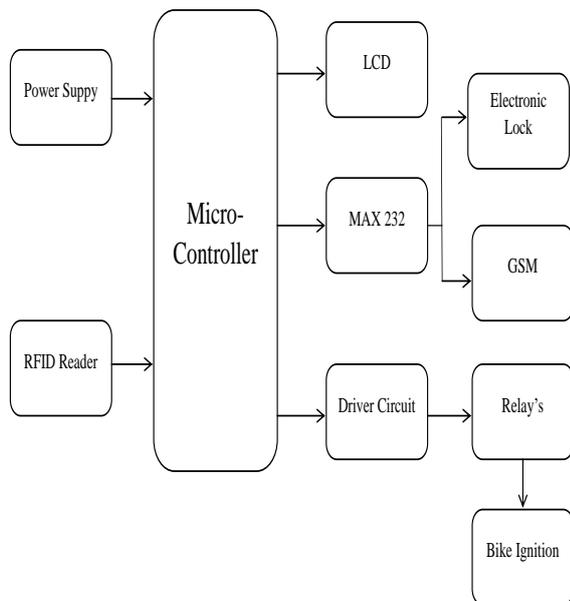
Fig2 schematic diagram of the system
