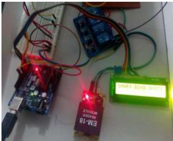
*Fig.3* Basic LCD display when bike start
