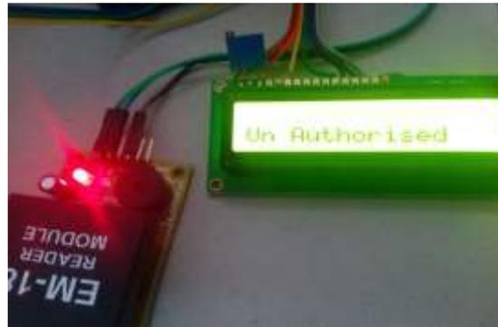
*Figure6:* When unauthorized person access the tag
