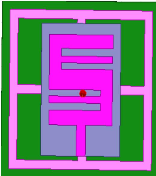
Figure 10. EBG Structure with inverted E antenna
