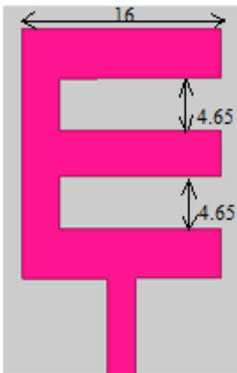
Figure 4.E Shaped Antenna
