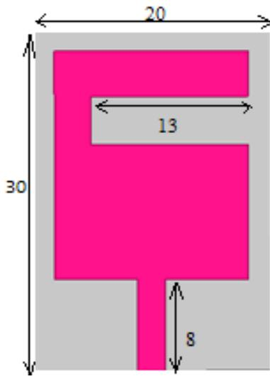
Figure 3. Patch with Upper Slot
