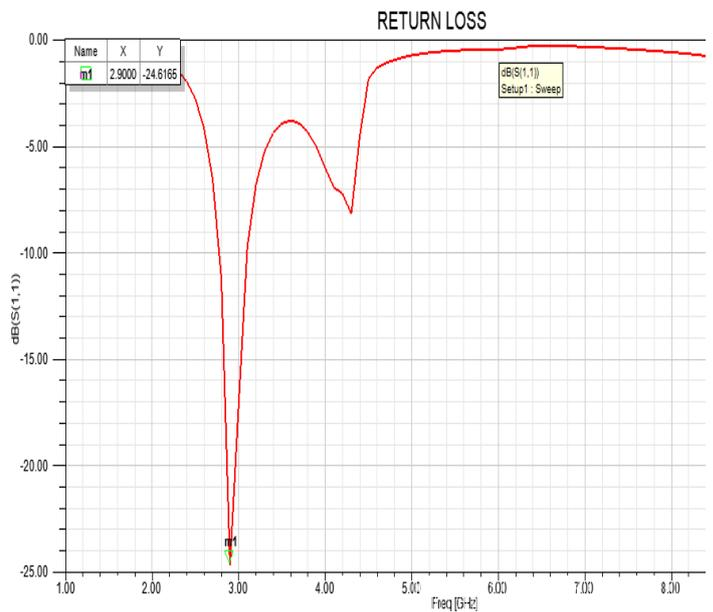
Figure 8. Return loss for inverted E shaped antenna
