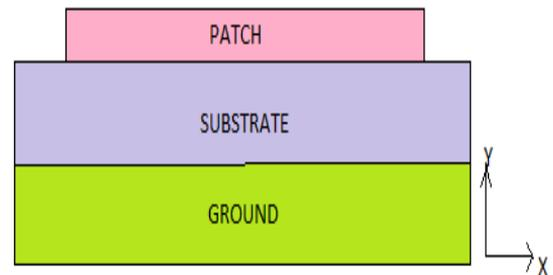
Figure 1. The basic antenna structure
