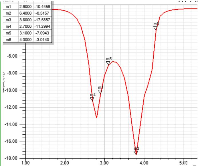
Figure 11. Return loss for EBG based inverted E structure
